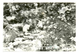
Fig. 1. Scanning electron micrograph of UMM. Cracks, flaws and continuous pores of larger sizes are apparent.
